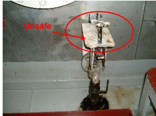
with his foot operating the valve lever. The improvised arrangement was fabricated to allow unmonitored draining of the HFO Settling Tank. In this particular case, upon completion of draining, the screw down T-bolt was presumably not turned back fully enough to allow the valve lever to return to the closed position, which caused the valve to drip.
